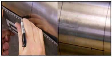
Figure 3-15: Marking the 9 o'Clock Position
